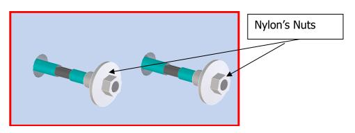
8 Move down the ceramic Hub up to lean on the elements fixing previously fixed to the wall
